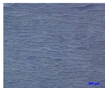
Microstructure obtained by SLM (after etching)
