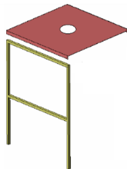
Figure 9 Assembling the top shelf
