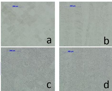
The microstructure obtained during SLM with Ti-6Al-4V is composed of acicular martensitic  $\alpha'$ -phase. The Z surface (a) shows long columnar grains which grow according to the build direction, while the XY surface (b) shows a checkerboard like surface, due to the laser strategy crossing at 90° between each layer. The pictures (c) and (d) show respectively the Z surface and the XY surface of the sample after heat treatment, the microstructure is composed of  $\alpha+\beta$  phase.
